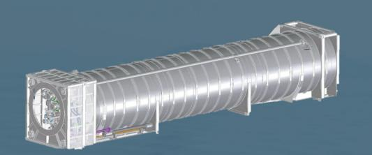
Design, build and test a prototype of an intermodal ISO 45 LH2 container and of its evaporator (by CHART). **Design and** test the tank connection space (to safely connect the container to the ship's power plant).
